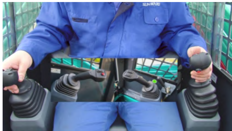
Operation with pilot handles
