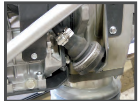
SPARK ARRESTOR OPTION - FOR USE IN ZONE 1 & 2 APPLICATIONS WHERE RISK OF IGNITION HAS TO BE SUPPRESSED
